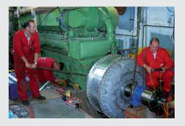
Misalignment is a main cause of machinery failure. Generally, misalignment is caused by inadequate measurement techniques, an improper foundation or degradation of the foundation. The alignment of a propulsion unit can also be influenced by deformations in a vessel's engine room and hull, caused by changes in the operation conditions, working environment or the cargo load condition
